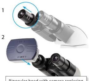
Binocular head with camera replacing the original eyepiece
